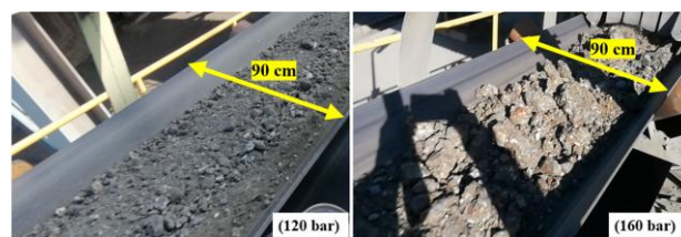
Fig.3. HPGR belt product in the operational pressures of 120 bar and 160 bar.
